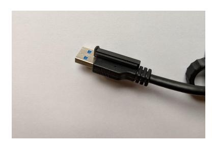
**Step 3:** Attach the second cable cover over the other half of the USB Cable.
