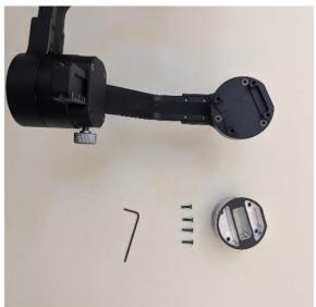
**Step 4:** Remove gimbal from camera arm with thumb screw.
