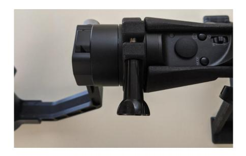
**Step 5:** Assemble camera mounting adapter with hub and arm.
