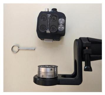
**Step 8:** Install pull pin with camera then reconnect USB and circular connectors.
