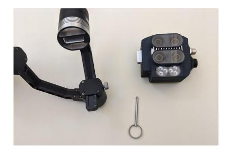
Step 3: Remove camera mounting adapter from gimbal. A 1.5mm hex wrench is required to remove the four screws retaining the adapter.
