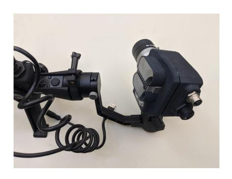
Step 2: Remove camera head from gimbal by removing pull pin.
